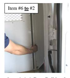
Loosely bolt **Rear Bulkhead Doorframe** (at the door hinge) to **Bench/Wall** assemblies using ½"
